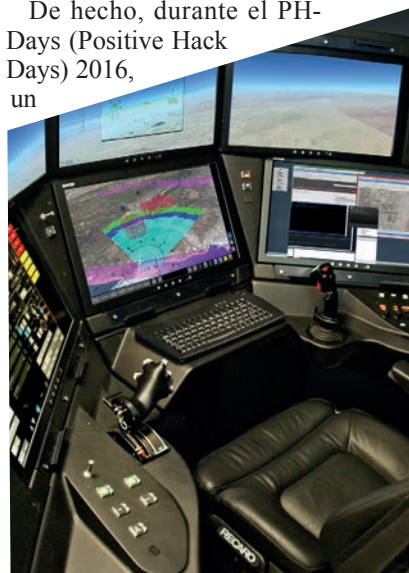
Advanced Cockpit GCS de General Atomics Aeronautical Systems.
