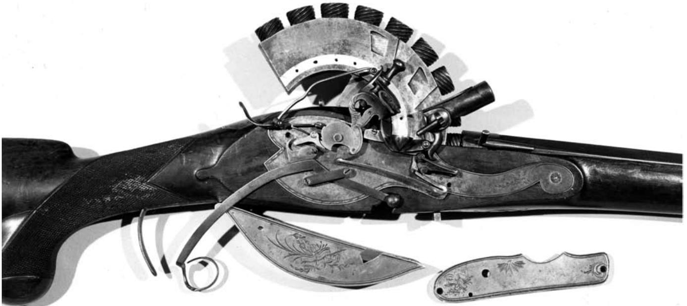
5. The lock mechanism with the cover plate removed.
