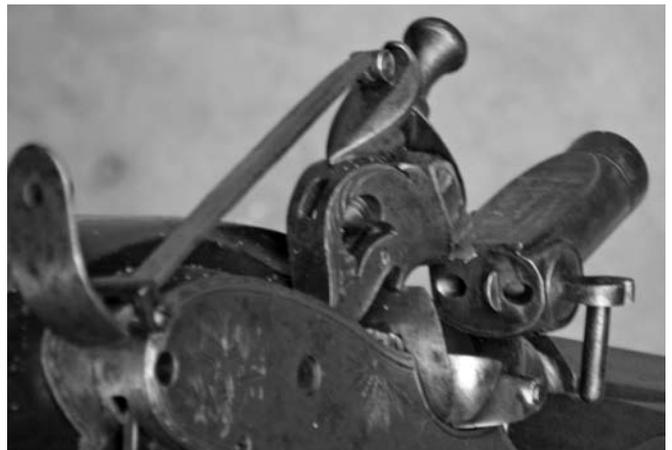
8. The priming magazine frizzle. Note the tap valve and on the underside the two holes separated by a semi-circular fence.
