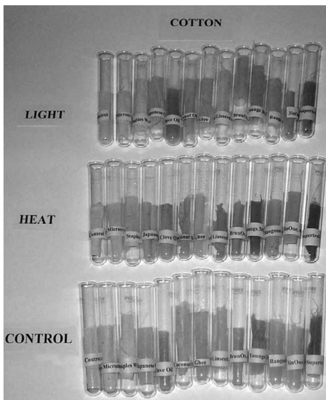
Figure 8: The effects of coatings on cotton after one month.
