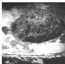
Figure 2: Corrosion of an iron screw caused by the deterioration of cellulose acetate. (Harrington & Richardson single grip post 1940, No accession number)
