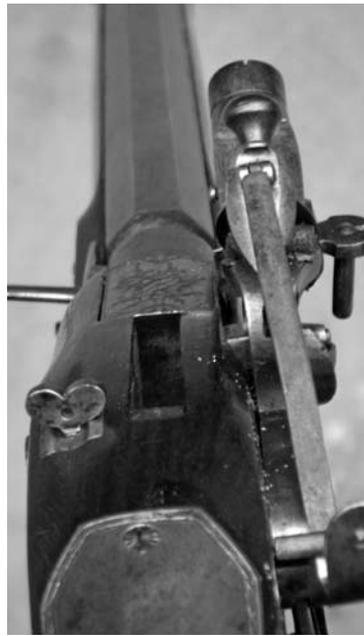
10. A firer's-eye view of the breech area of the rifle when preparing to fire. Note the offset peep-sight on the left.
