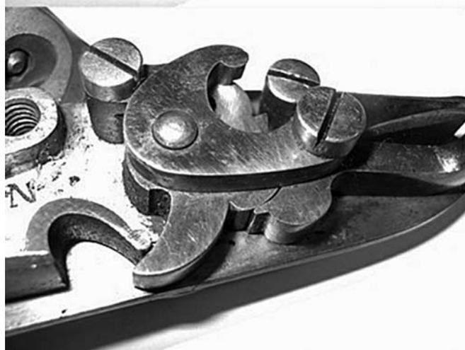
internal views of the same locks – the major difference is the lack of any assembly marks/numbers on le Blanc's lock (bottom)
