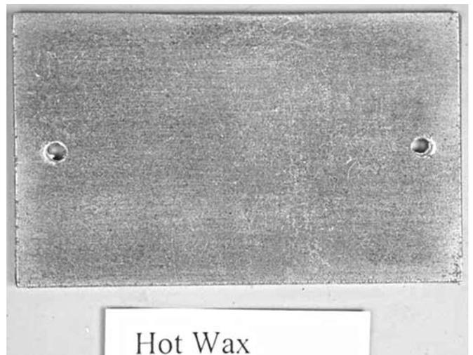
Figure 13: Mild steel coupon treated with hot Renaissance Micro-crystalline wax.
