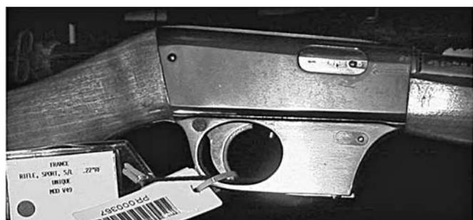
Figure 3: French sporting rifle with metal surface keyed to take a coating.
