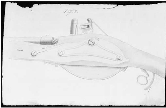
17. An original drawing of the nearside of the breech area of the "poli-chambered" rifle.
