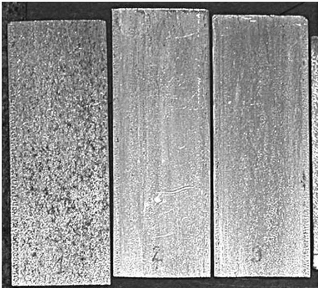
Figure 9: Mild Steel coupons coated with, (left to right) untreated, Paraloid B72, Renaissance Micro-crystalline wax kept in a showcase.
