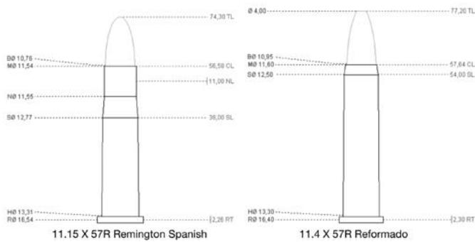
Figure 2. Dimensions of the .43 Spanish and Reformado cartridges.
