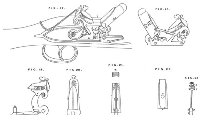
14. Sheet 3 of Thomson's patent illustrations (Figs. 17 to 23); an automatically-priming lock.
