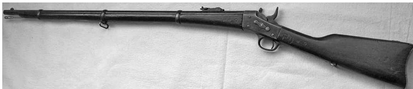
Figure 1. The well-worn 3rd contract Remington-manufactured No.1-model Rolling Block rifle (Remington model 71) in .43 Spanish calibre found to have disappointing accuracy. Replacement cleaning rod and rear sling swivel courtesy of Kenn Womack.
