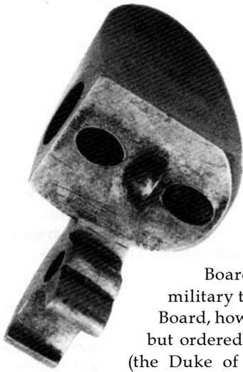
23. The underside of the priming magazine "hammer" of the musket in Figure 22, showing the two powder holes divided by a semicircular fence.
