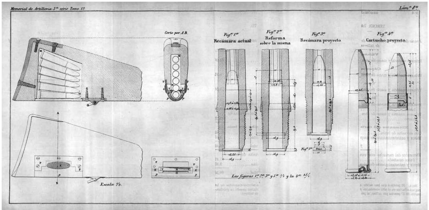
Figure 3. Original diagram of proposed modification of .43 Spanish rifle to Reformado.
