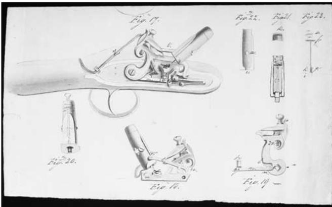
18. Original drawings for Thomson's design for an automatically-priming lock.
