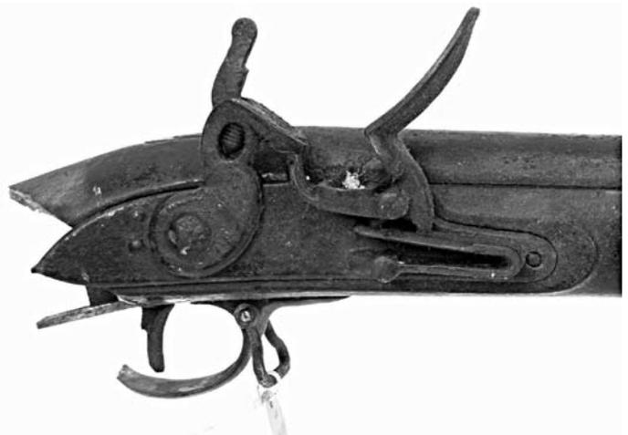
Figure 1: Moving parts of a firearm fixed due to application of a coating.
