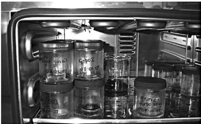
Figure 5: Material testing jars placed in the incubator.
