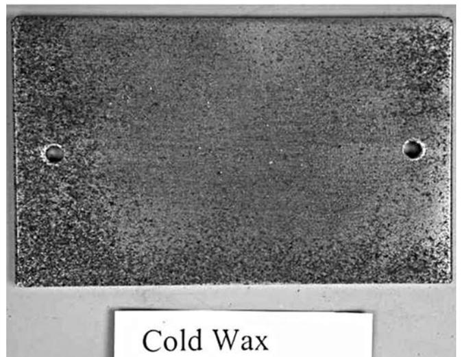
Figure 12: Mild steel coupon treated with cold Renaissance Micro-crystalline wax.
