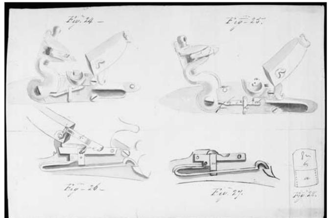
20. Original drawings for Thomson's two designs for constricted breeches to reduce the loading time of service muskets.
