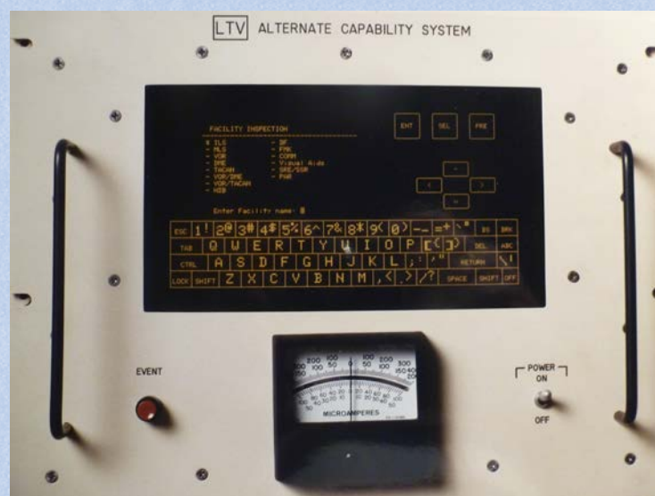
Sistema ACS (Alternate Capability System) alternativo a la consola principal
