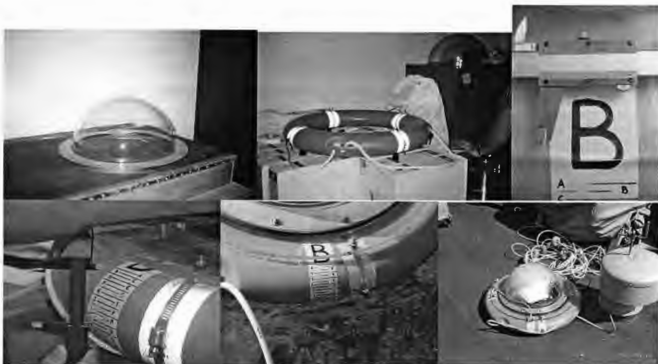
Fig. 31: Sequence of ensambling the wave-rider GPS buoy used in the 2000 experiment, calibration and the buoy on board of the boat.
