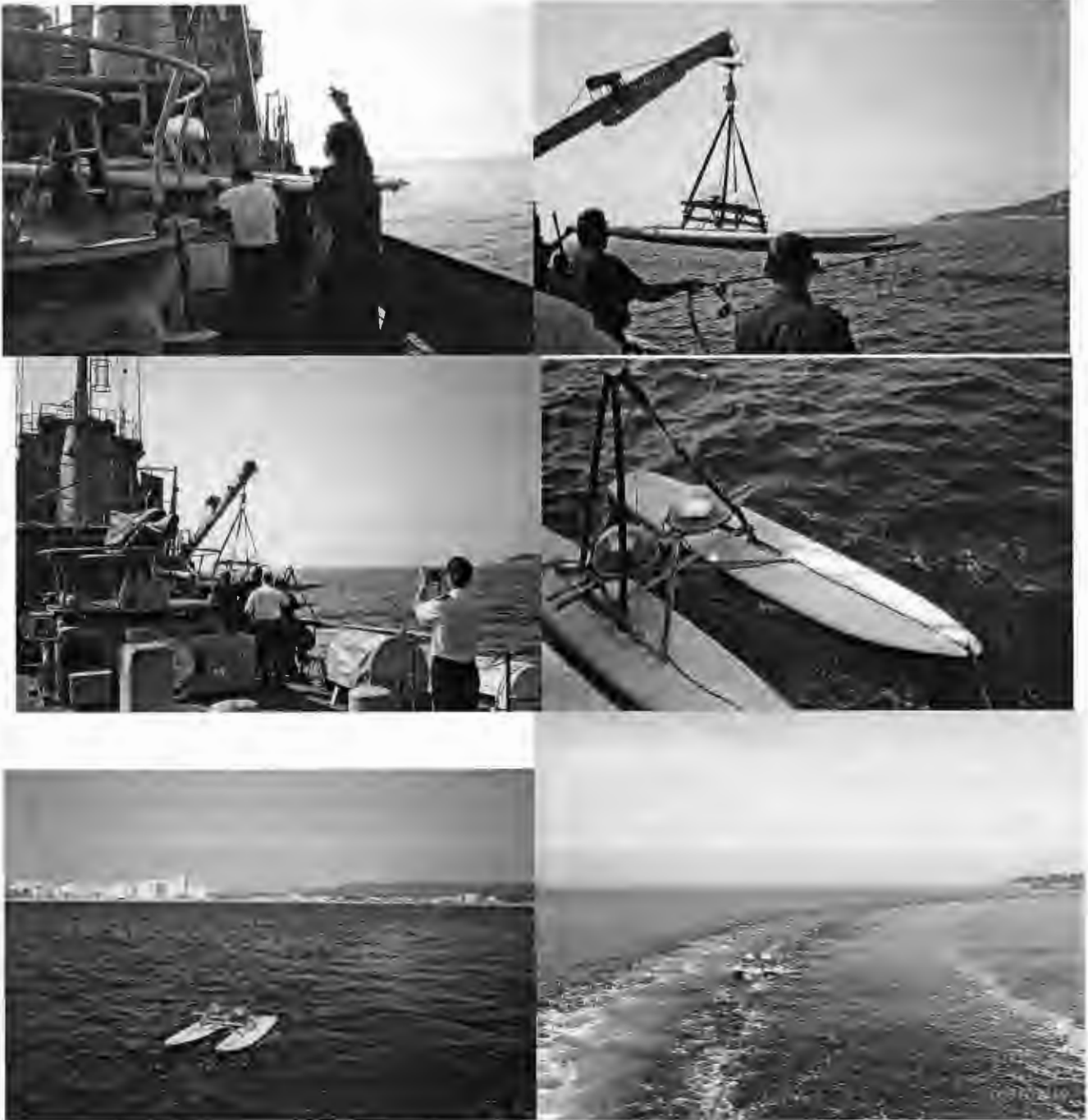
Fig. 34: Set of pictures showing the design and use of the GPS catamaran
