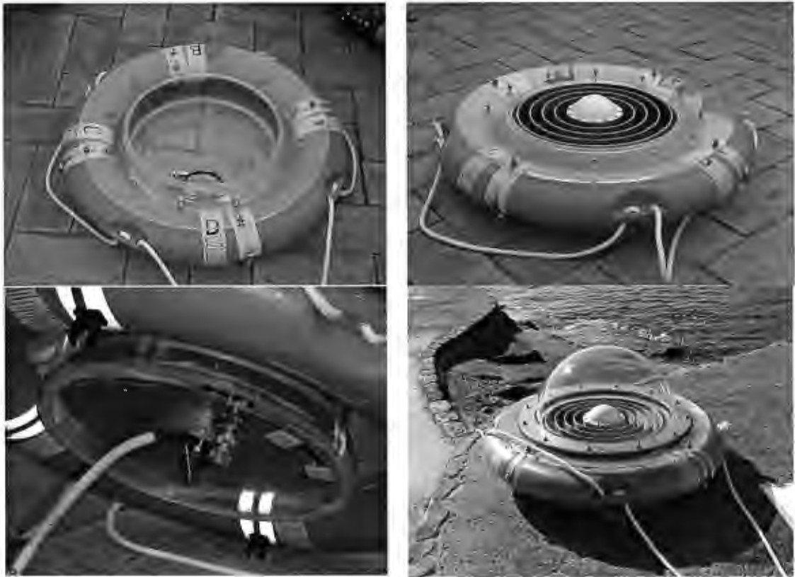
Fig. 80: Sequence of ensambling the wave-raider GPS buoy used in the 2000 experiment.
