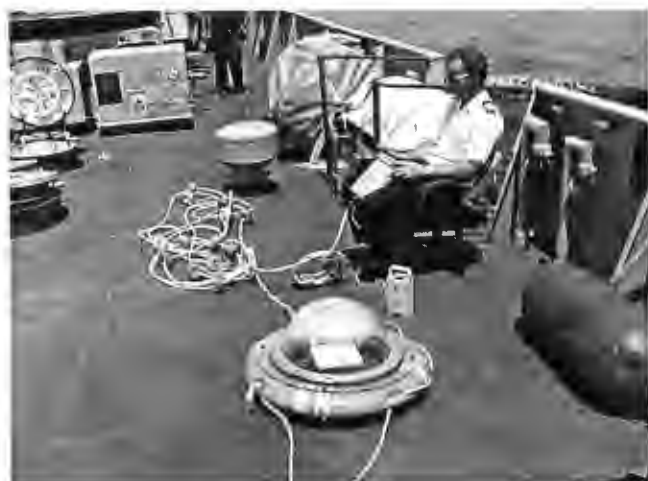
Fig. 53: Verification of good GPS receiver data from catamaran
