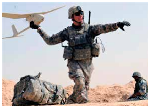
An RQ-11B Raven, an SUAS employed by 2/2 Cav, is launched by a Soldier in Iraq. (U.S. Army photo)
