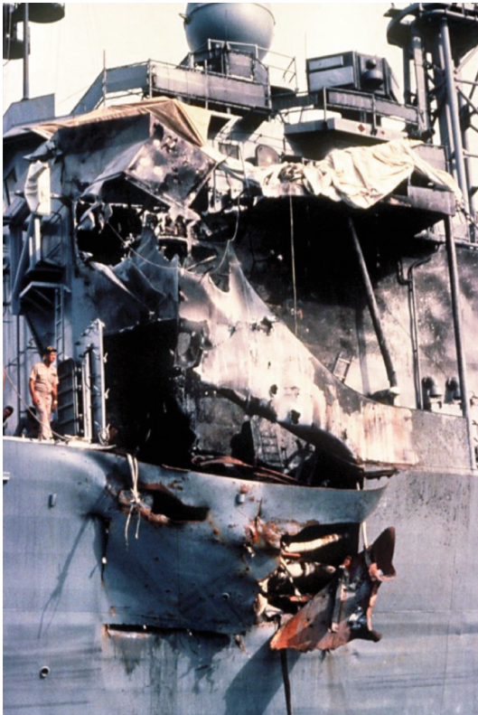
USS Stark. Detalle de los daños externos. (Foto: USS Stark. US Navy photo DVID #DN-ST-89-01563 from NavSource. Photographic History of the US Navy: NavSource. www.navsource.org ).
