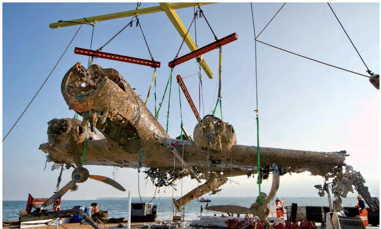
The biggest problem to overcome was how to lift an object that is delicate without causing too much damage. Discussions took place, and it was decided that the best way forward was to build a framework round the aircraft, lift out the framework without attaching it to the aircraft, therefore no additional stress was applied to the delicate object.
