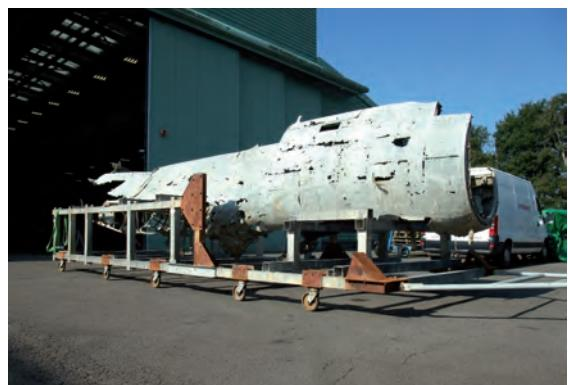
copies of the Dornier Air Publications allowing them to reference possible areas for lifting the aircraft. Areas inside the bomb-bay and around the undercarriage attachments to the spars were identified with this information being sent to the dive team.
